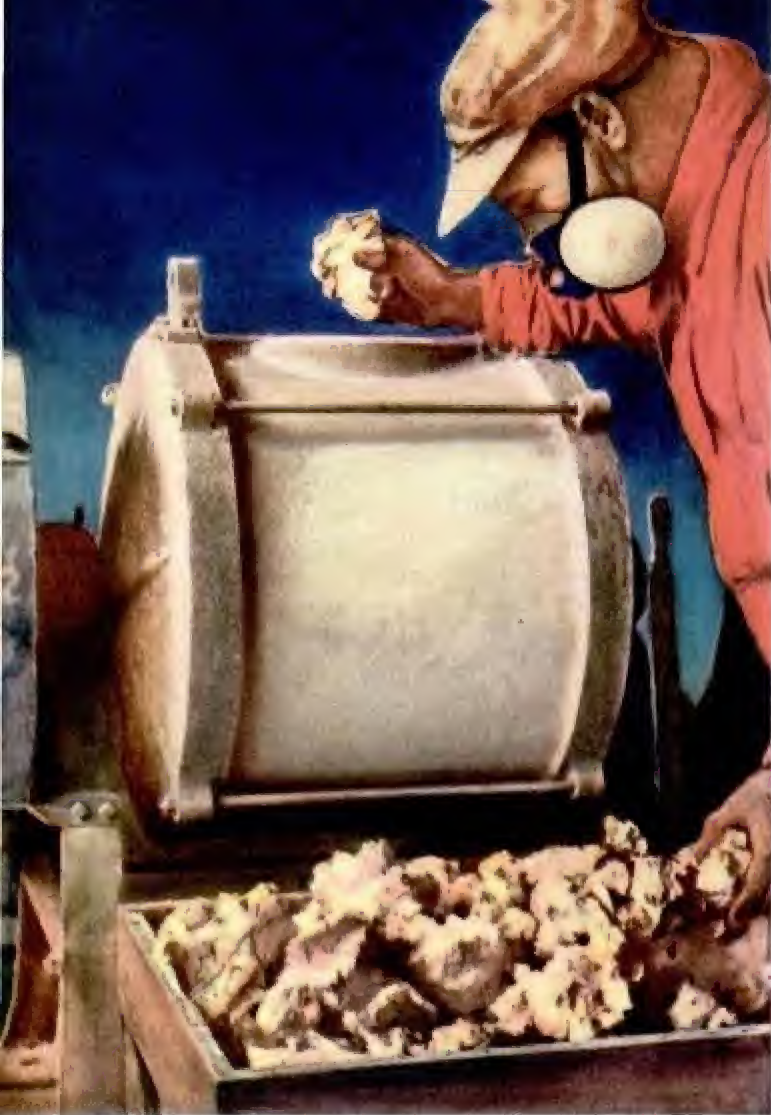
Grinding sodium uranate, a heavy, bright yellow, clay-like substance to be used as pigment. This is a common form of uranium, heaviest element and parent of radium
